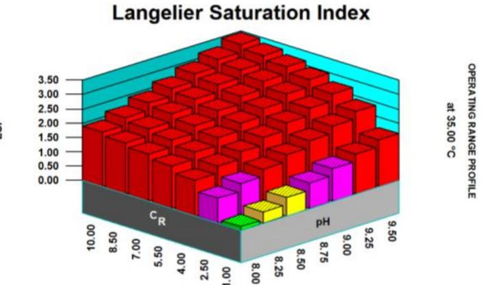
\*\* It shown that, pH higher 8, cycle higher 4, at 35 deg. C of cooling tower water, very high tendency to scale\*\*
