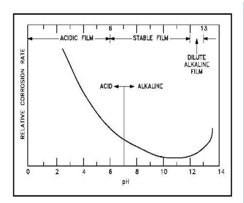
High pH , low corrosion rate
